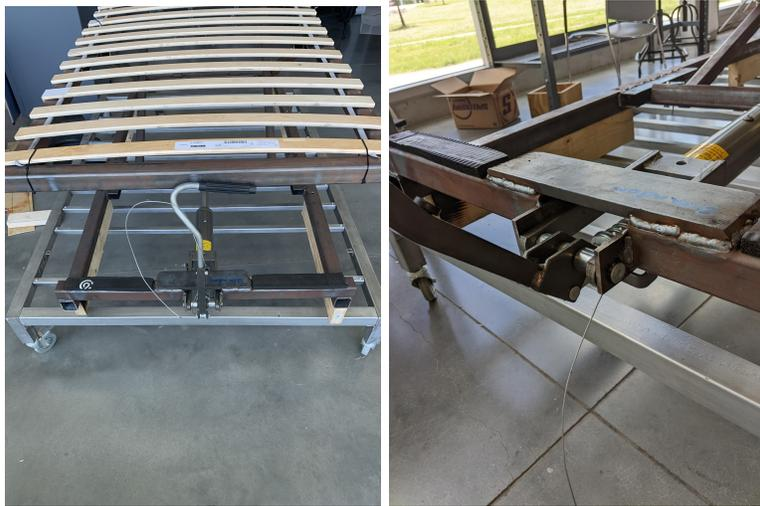
Images showing the required modifications to the back of the device to accommodate the hydraulic.
