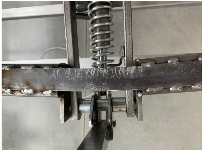
First image shows team member Paxton Neff supported by the assembled device during initial testing. Second image shows the 1/8" piece of steel that was originally welded over the gap in the bottom frame along with the noticeable bend and deformation after testing concluded. This part was cut off and a larger, ½" thick plate was welded in its place.
