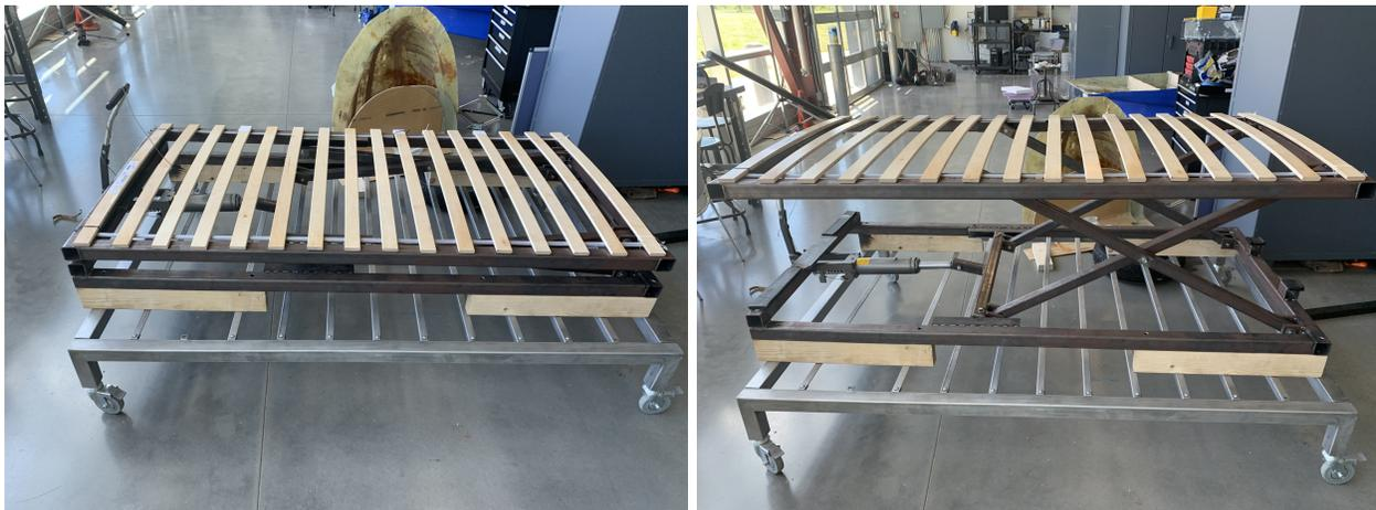
Fully assembled device in both the raised and lowered positions. Note the bed frame used was for a full sized bed, rather than a twin.
