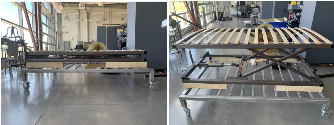
Side view of the device lowered and fully raised, note the aforementioned spacers, supports, and padding present on the bottom frame.
