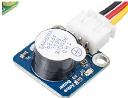
Figure 7: Active Piezo Buzzer
