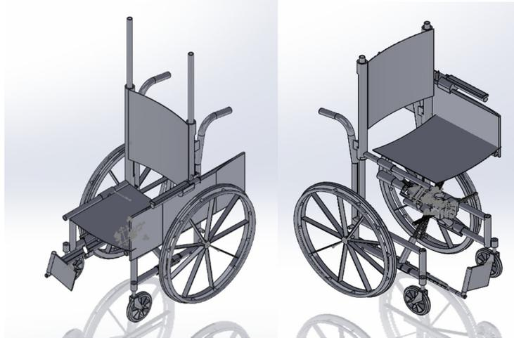
Figure 1 and 2: Comprehensive model with seat raised and lowered
