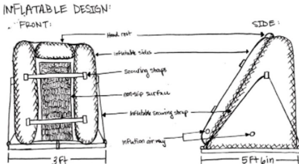
The team chose a design with progressive inflation. First the backboard surface directly supporting the subject would be inflated to create a “rigid” surface that would then be lifted by multiple wedges in the inflatable.
