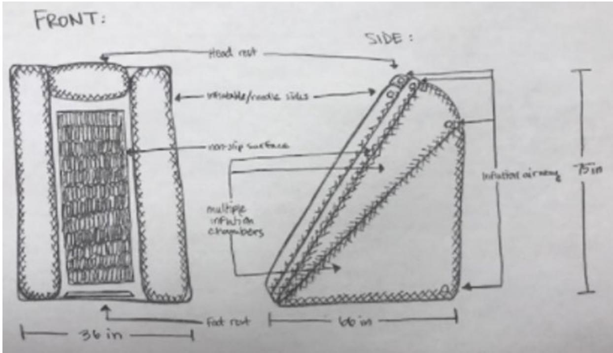
In testing they found that the inflatable backboard would easily buckle/fold during inflation of the wedges, so the team opted for a semi-rigid backboard made of lightweight foam. This improved the performance. And the team finalized the design and sent it out for fabrication.
