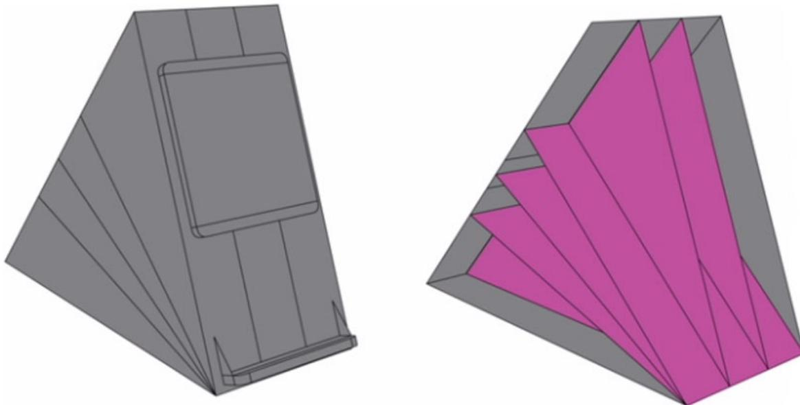
*Computer-Aided Design of the inflatable (outside shown left, and internal baffles shown right).*
