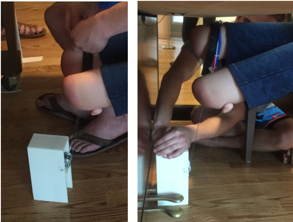
Fig. 2. Student attaches pulley lines to leg cuff (left) and Heidi plays using the pulley system pedal pusher (right). The student holds the pusher box down for the prototype, but this would be resisted by an extension to the keyboard.
