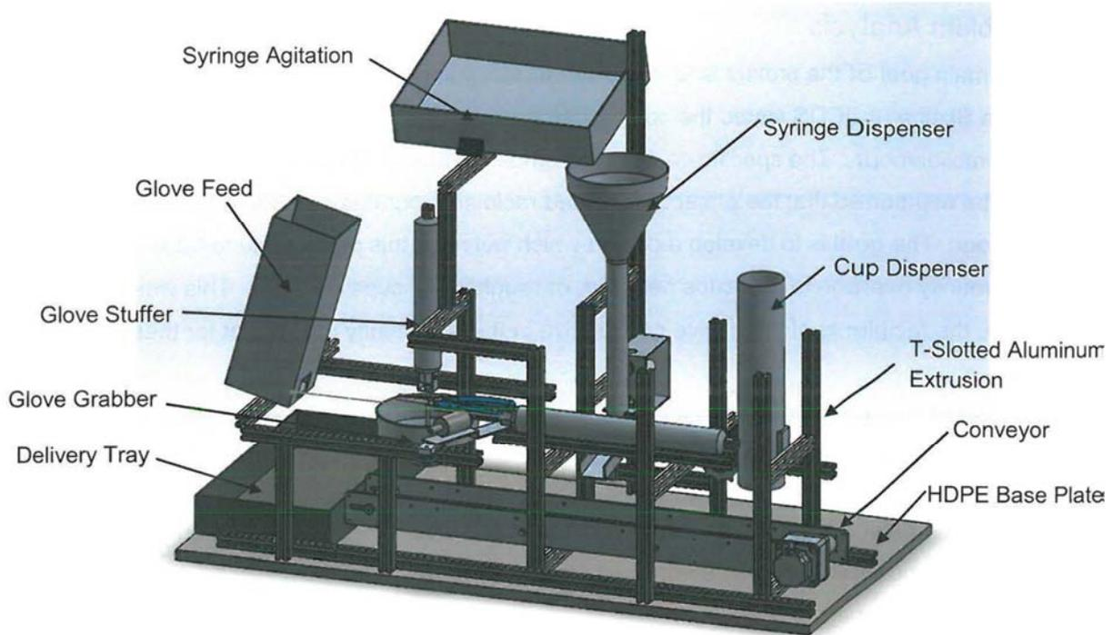
Figure 3: CAD Model of Full Packaging Assembly
