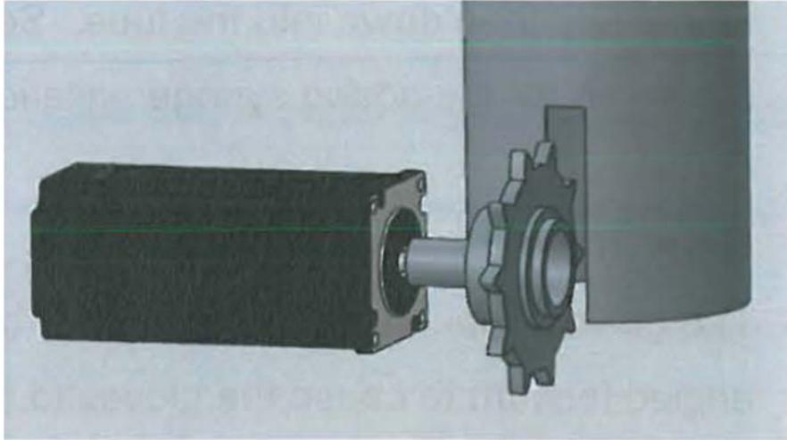
Figure 4: Cup dispenser with stepper motor/sprocket design
