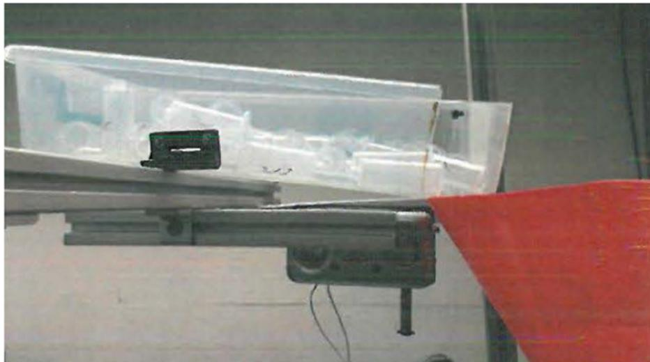
Figure 5: Syringe bin with agitation system to feed syringes to funnel and dispensing tube.
