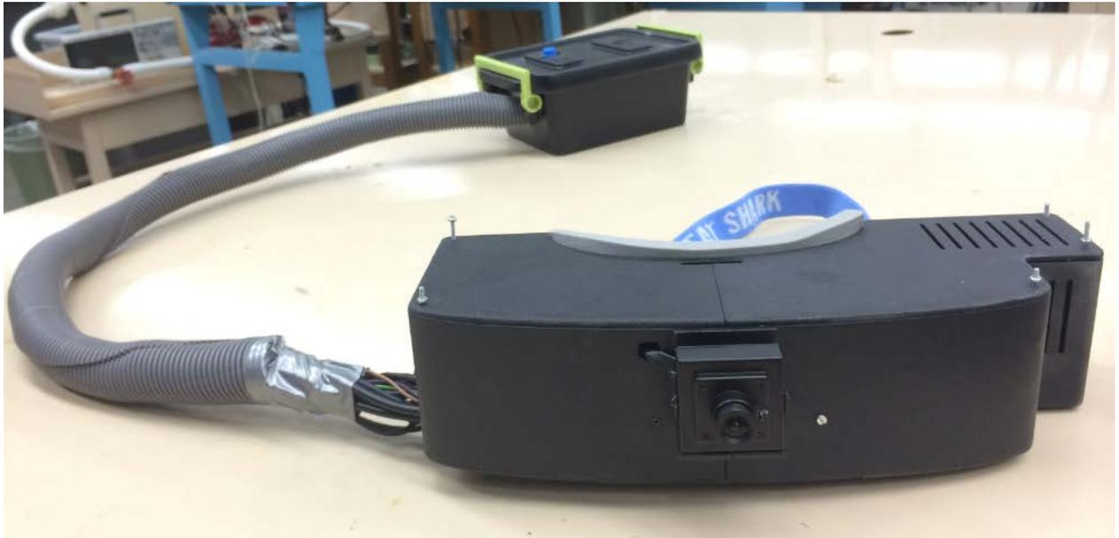
**Figure 5.31: Computer Vision Compensator Version 3.0 Prototype. All components were set up in the device.**
