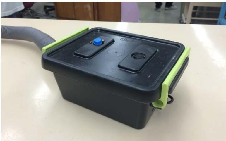
**Figure 5.30: Control Box Prototype. The black switch is the power switch, and the blue button is the calibration.**
