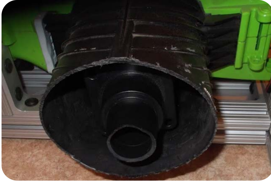
Figure 2. One step reducer from a 5 inch tube to a 1.5 inch tube.
