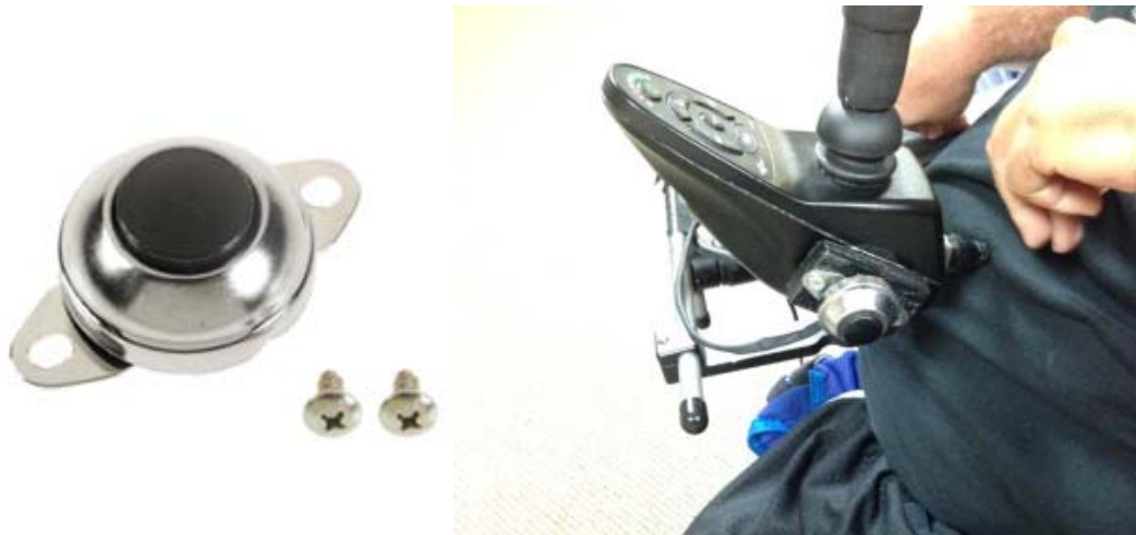
Figure 6. Low-force momentary switch (left) for powering the vacuum unit on and off (mounted, right).
