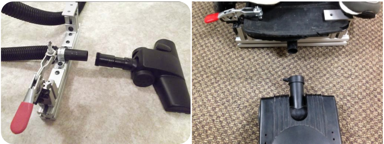
Figure 5. Nozzle mounting system (left) for attachment to the wheelchair footrests (right).
