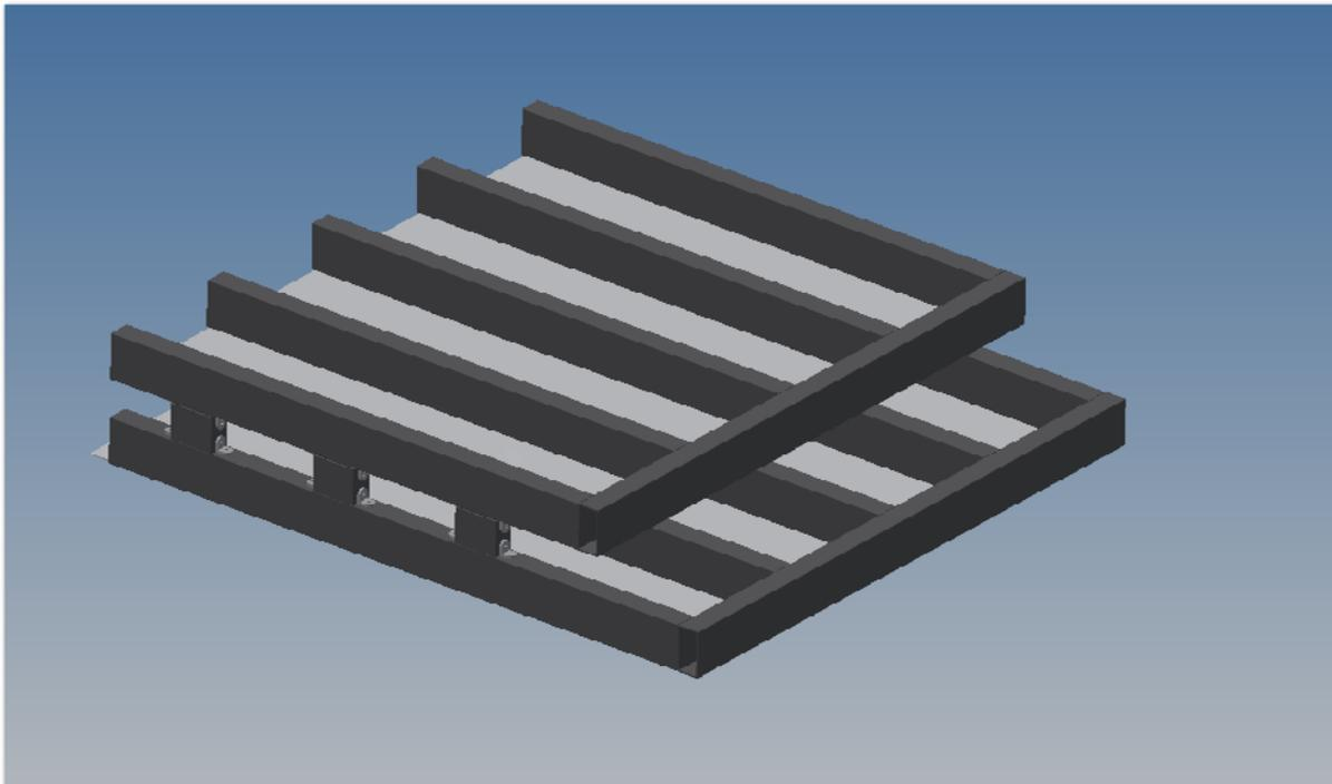
Figure 4. Strap Delivery Device
