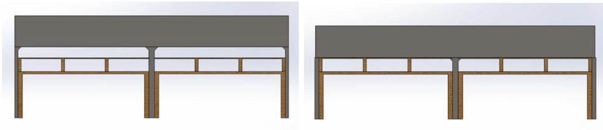
Figure 2. Conveyor height reduction from the original (left) to the final (right).
