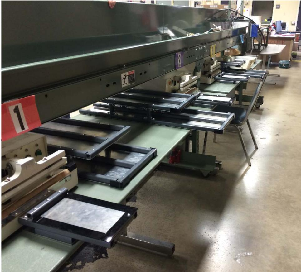
Figure 5. Heat sealing line with all modifications.
