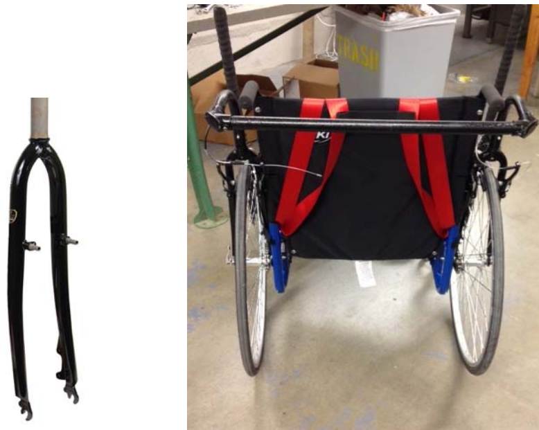
Figure 1: Chromoly Steel Bike Fork (left) and Bike Forks on Wheelchair with the Anti-Rotation Support Bar Structure Connecting them.
